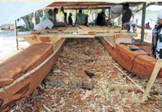
New drua in the making at Fulaga. Right: Sail weaving for the new drua. Photo: Carol Dunlop
